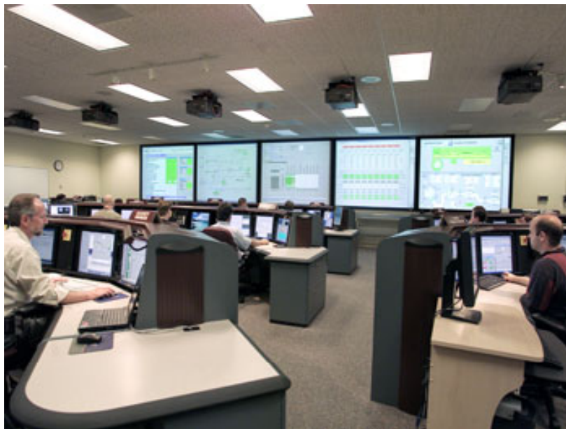
Figure 3. Operators in the NIF Control Room can continuously track data generated by the integrated computer control system on their monitors. The Shot Director's station is on the left.
