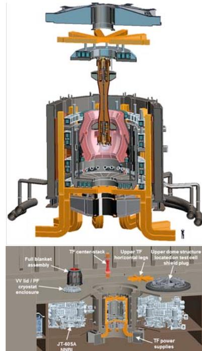
**Figure 2** – (Top) Cross-section of  $R_0 = 1.7$ m ST-FNSF showing vertical maintenance strategy, (bottom) example layout of test-cell and components during maintenance.
