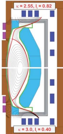
**Figure 1** -  $R_0 = 1.7m$  ST-FNSF: TF coils (brown), divertor / outboard PF coils (purple / dark blue), vessel and shielding (gray), breeding blankets (light blue), limiter outline (green), and plasma poloidal flux contours (black and red). Upper / lower plots are  $l_i = 0.82 / 0.40$  and  $\kappa = 2.55 / 3.0$ .
