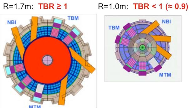
Figure 3 – Side-by-side comparison of mid-plane sections of  $R_0=1.7$ m and 1m ST-FNSF devices showing TBR and TBM, MTM, and NBI ports.
