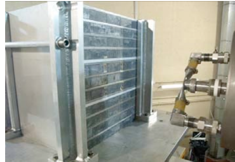
Fig. 1b. HCLL mock-up assembled in front of FNG target.
