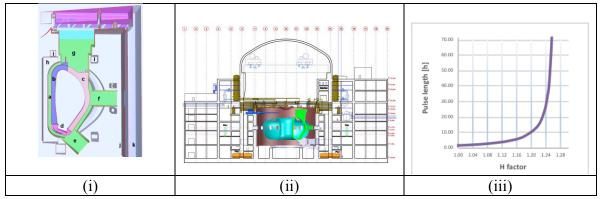
Fig. 2: (i) Tokamak elevation build: a) vacuum-vessel; breeding blanket (inboard); c) breeding blanket (outboard); d) divertor; e) lower port; f (equatorial port; g) upper port; h) toroidal field coils; i) poloidal field coils; j) cryostat; k) bioshield; (ii) DEMO tokamak building complex; and (iii) Pulse length as a function of the H factor for the alternative scenario Flexi-DEMO.
